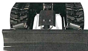
Retracted undercarriage : 955 mm
