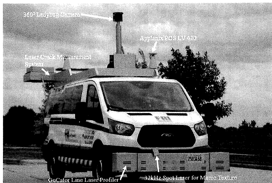
Figure 1: ERI's Automated 3D Pavement Data Collection Vehicle System
