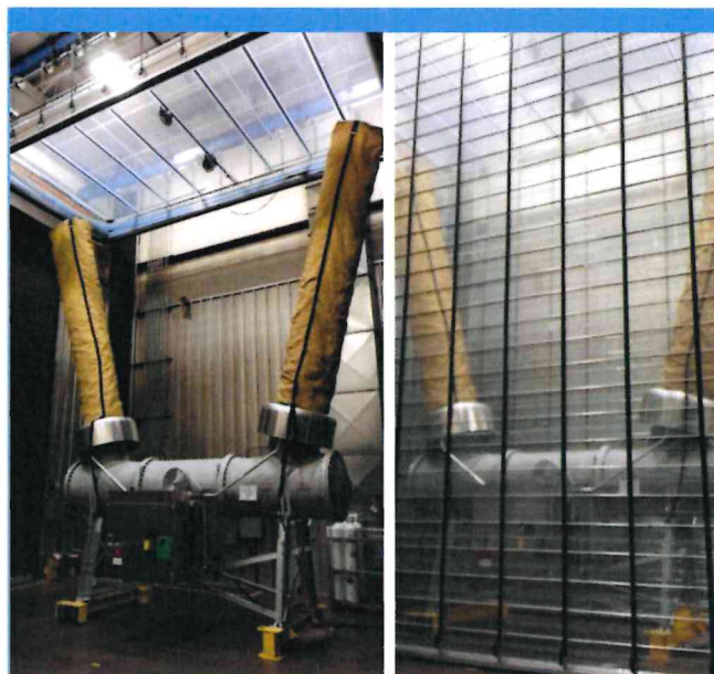
550 kV Dead Tank Volumetric Tightness Testing
