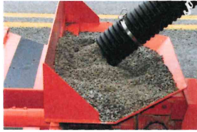
Gravity Feed Aggregate Delivery
